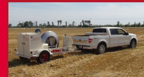
Field operating speeds typically vary from 8 to 12 mph, depending on field conditions. On the road, the Falcon can be towed at normal speeds
