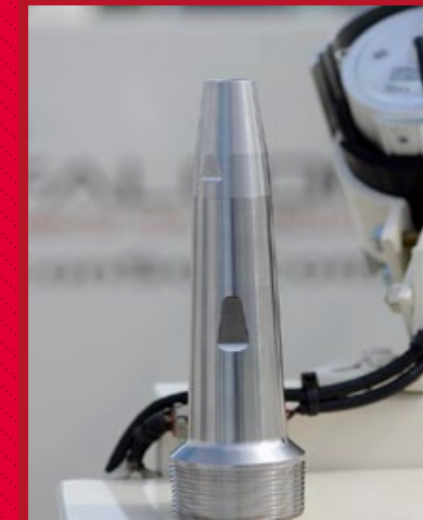
Depending on the desired core depth, a 4" to 12" cone-tipped stainless steel probe with a replaceable tip collects and deposits a soil core into the stainless drum with every revolution
