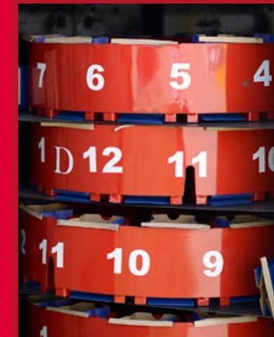
13 on-board carousels allow 156 samples to be collected before refilling
