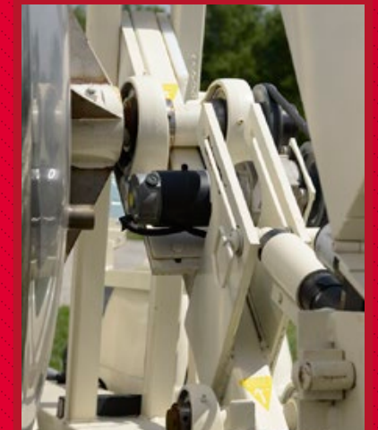
When the user-defined core count is achieved, a 12-volt motor raises and rotates the drum to assure proper mixing as the Falcon drives to the next sampling site
