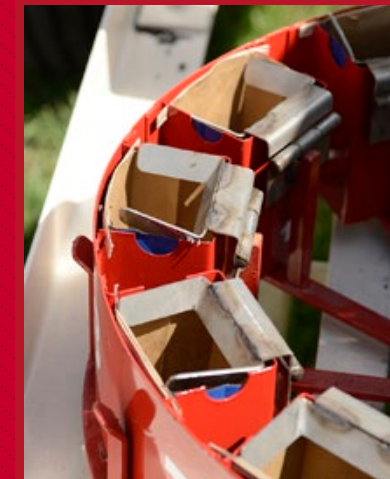
A stainless steel funnel is lowered to fill the mixed sample into a pre-labeled sample bag in a 12-position keyed carousel
