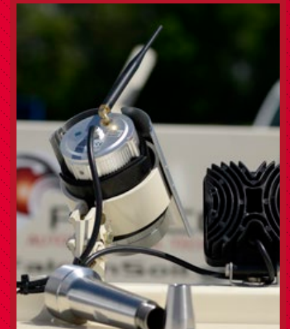
To allow the operator to monitor operations, a wireless illuminated camera streams video to a laptop computer in the tow vehicle
